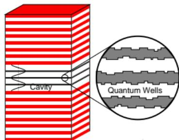
$$H = \omega\psi^\dagger\psi + \sum_i \omega_0 S_i^z + g(\psi S_i^+ + \text{H.c.})$$
