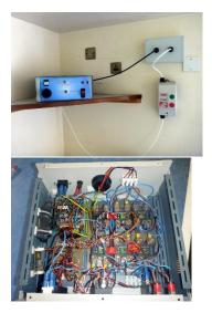
This system controls the rotation and opening/closing of the domes at the Napier building of the observatory.
