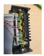
Pictured on the left here is a 10 channel, high bandwidth transimpedance amplifier with high current output to drive oleds.
