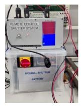
This system to the left is a remote-controlled shutter driver for the heavy shutter for the Gregory telescope. Currents of greater than 50A had to be delivered to the high-powered
